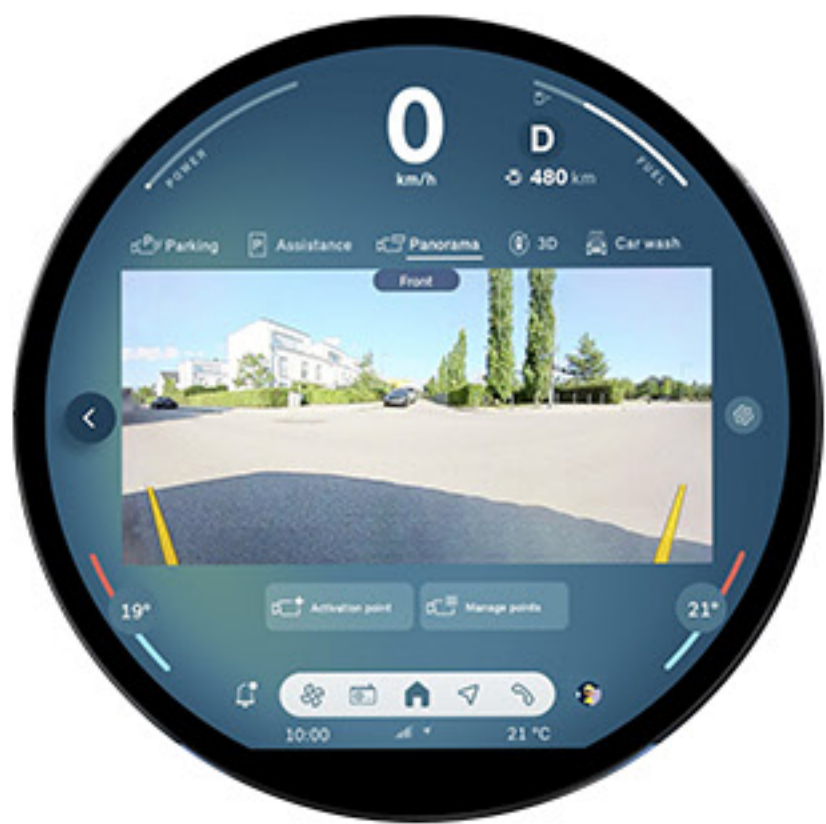
Parking assistant: Visual parking aid featuring rear view camera, makes parallel and perpendicular parking on the road easier. The system completely takes over the steering, the accelerator, and the transmission.
